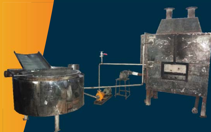
CIRCULAR FRYER WITH WOOD FIRED EXTERNAL HEAT EXCHANGER
